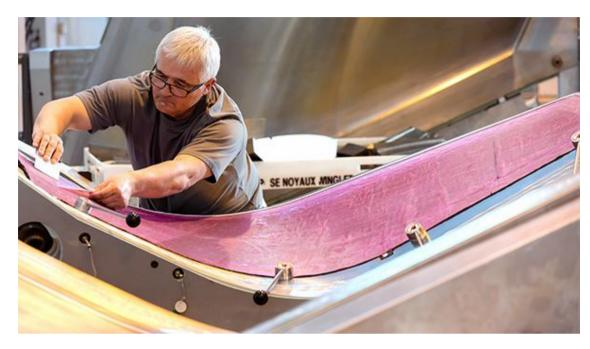
The use of composites has been consistently growing for structural parts, such as the Dassault Falcon 8X business jet's winglets.
